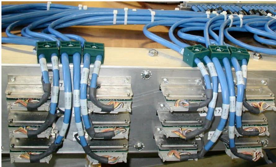
Figure 5: A view of the anode front-end boards installed on a chamber. Also shown are the AFEB-ALCT cables.
