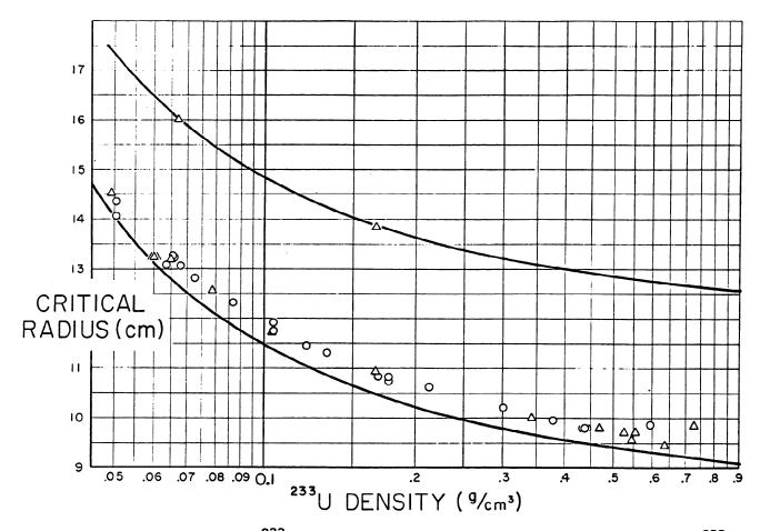
Fig. 13. Critical radii for  $^{233}$ U metal-water spheres, bare and water-reflected, vs  $^{233}$ U density. The experimental data are described in References 53 - 56 while the solid line is theoretical. Unreflected experiments are few, and the theory is disappointingly low for the water-reflected cores.
