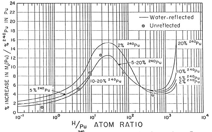
Fig. 17. Computed influence of  $^{240}$ Pu on the critical mass of metal-water spheres. The solid lines are from Roach<sup>(13)</sup> and represent reflected spheres. The points are for bare systems and were calculated by G. I. Bell and C. B. Mills<sup>(14)</sup> with an 18-group cross section set and the DSN transport code.
