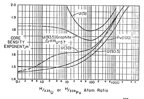
Fig. 3. Core density exponents for several materials vs the  ${\rm H}/{^{235}{\rm U}}$  or  ${\rm H}/{^{239}{\rm Pu}}$  atom ratio. The reflector is thick water at normal density in all cases.
