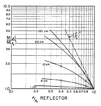
Fig. 25. Computed critical masses for U(93.5)-graphite cores (C/235U = 17.77) as a function of graphite reflector density.
