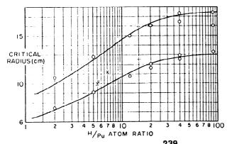
Fig. 16. Critical radii vs  $H/^{239}$ Pu atom ratio for bare and lucite-reflected cores of plutonium metal-lucite mixtures. Experiments employing different materials were adjusted to this mixture. Symbols are defined in the caption for Fig. 15. The solid line is theoretical.
