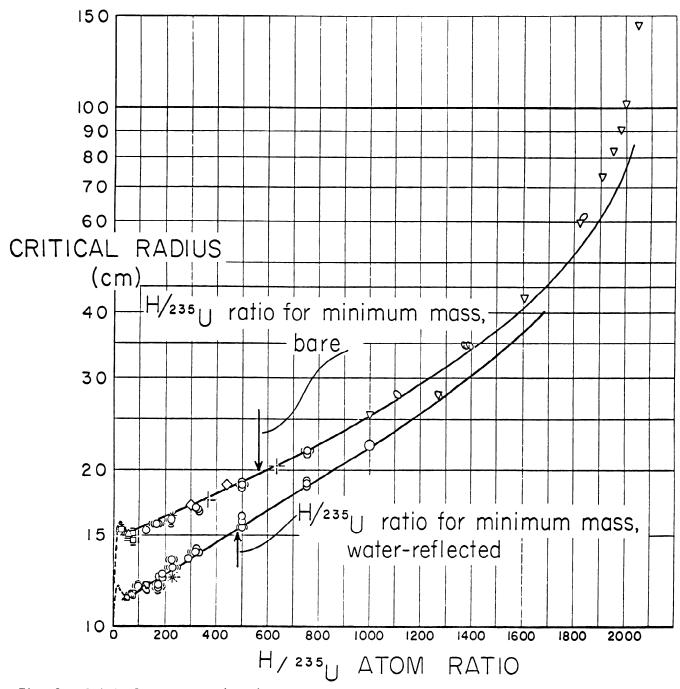
Fig. 9. Critical radii of  $U(93.5)0_{2}F_{2}$  water solutions, bare and water-reflected, vs the H/235U atom ratio. The solid line represents the results of theory. Symbols are defined in the caption for Fig. 8.
