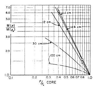
Fig. 24. Computed critical masses for U(93.5)-graphite cores (C/235U = 17.77) as a function of core density for five thicknesses of graphite reflector. Core density exponents may be derived from this figure, but note that for thick reflectors the exponent will not be a constant.
