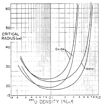
Fig. 11. Theoretical critical radii for U(5) metal-water and  $U(5)O_2$ -water spheres vs 235U density. Direct comparison to experiments for this enrichment is in Tables IX and X.
