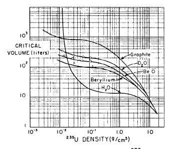
Fig. 19. Bare critical volume vs  $^{235}$ U density for several U(93.5) metal moderator mixtures. The data for water and graphite are taken from Table V while those for Be, BeO, and D<sub>2</sub>O are due to C. B. Mills.(69) For all metal-moderator mixtures, the critical volume increases monotonically with decreasing  $^{235}$ U density.
