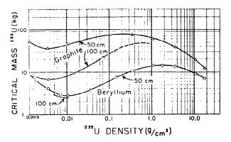
Fig. 26. Computed critical masses of U(93.5) metal reflected by thick graphite or beryllium for a wide range of  $2^{35}U$  densities. Note that these systems can be critically unstable in the region in which critical mass decreases with decreasing density.
