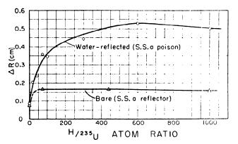
Fig. 6. Radius change for removal of a 1/16-in. stainless steel container as a function of the  $H/^{235}U$  atom ratio.
