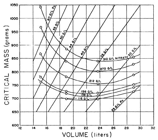
Fig. 18. Critical mass of water-reflected  $PuO_2(NO_3)_2$  spheres vs volume for varying amounts of excess HNO<sub>3</sub>. The 240Pu content was 3.12%, and the spheres include a 1/16-in.-stainless steel sphere.
