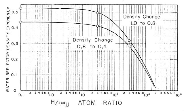
Fig. 4. Water reflector density exponents vs the core H/235U atom ratio for water-reflected, water-moderated spheres. As the reflector exponent is dependent upon the magnitude of the reflector density, the function is illustrated for two changes of density.
