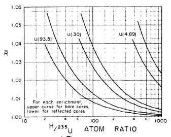
Fig. 5. Ratio ( $\blacksquare \overline{R}$ ) of uranium metal-water sphere radius to the UO<sub>2</sub>F<sub>2</sub> solution radius with densities appropriate to those of the solution vs the H/<sup>235</sup>U atom ratio. This uranium density is invariably less than that for the ideal metal-water mixture.
