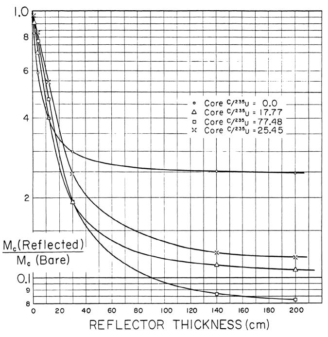
Fig. 20. Calculated ratio of graphite-reflected to bare critical masses for four core mixtures as a function of graphite reflector thickness. For the larger cores, up to 2 meters thickness is required for reflector saturation.
