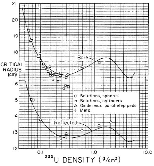
Fig. 10. Critical radii for U(30) metal-water cores, bare and water-reflected, vs  $^{235}\mathrm{U}$  densities.
