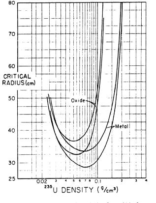
Fig. 12. Theoretical critical radii for U(2) metal-water and U(2)O<sub>2</sub>-water spheres, bare and water-reflected, vs  $2^{35}$ U density. Comparison to experiment is given in Table XIII.
