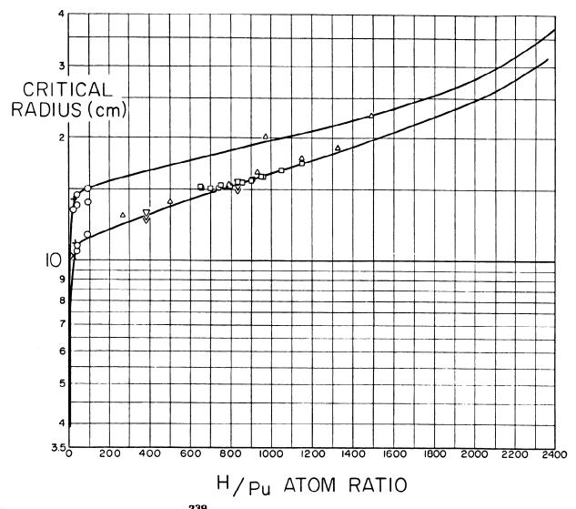
Fig. 15. Critical radii for <sup>239</sup>Pu metal-water spheres, bare and water-reflected, vs the  $H/^{239}$ Pu atom ratio. Symbols and references for this figure and for Fig. 16 are:  $\triangle$ , 57;  $\nabla$ , 58;  $\Box$ , 59, 60; X, 43; -1, 27. The solid line is theoretical.
