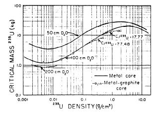
Fig. 27. Computed critical masses of U(93.5) metal and U(93.5) metal-graphite cores surrounded by three thicknesses of  $D_2O$ . At sufficiently low densities, the core graphite has little influence on critical mass. The instability mentioned in the caption for Fig. 26 also pertains to the systems of this figure.
