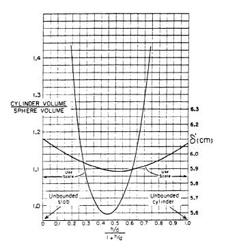
Fig. 1. (Cylinder volume)/(sphere volume) and  $\delta'$  = (extrapolation distance plus reflector saving) as functions of the dimensionless shape parameter  $\frac{h}{d}/(1+h/d)$  for water\_reflected, metal-water systems whose H/235U moderation ratio is about 30. These data were generated by application of the two-dimensional, as well as the one-dimensional, transport code.
