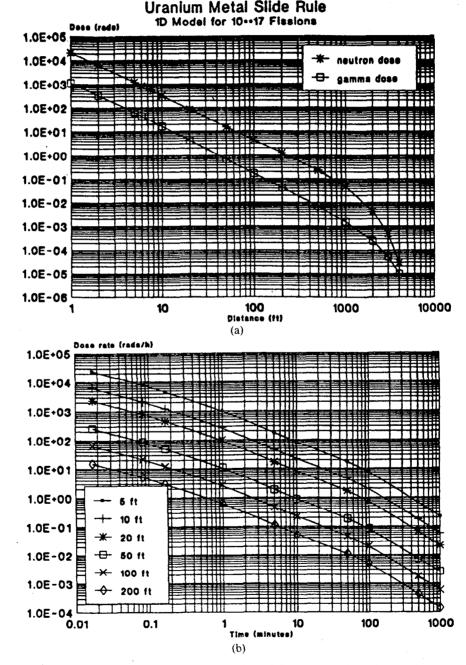
Fig. 1. Slide rule for U(93.2) metal: (a) prompt dose as a function of distance and (b) fission product gamma dose rate as a function of elapsed time.
