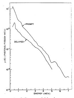
FIG. 5. Prompt and delayed  $\gamma$ -spectra.
