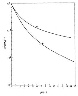
FIG. 3. Sphere transmission factors for an exponential attenuation kernel. Curve A is for a source distributed as  $1/4\pi r_0^{2r} (\sin \pi r/r_0)$ . Curve B is for a uniform source distribution.
