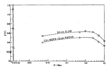
FIG. 1. Thermal neutron capture probability in a phantom.
