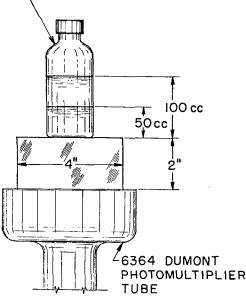
FIG. 7. Geometry of the blood counter.
