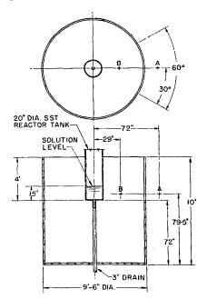
FIG. 6. Schematic of mock-up experiment.
