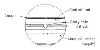
Fig. 7. Jezebel Pu (20% <sup>240</sup>Pu). Critical with insert in place, 5 lower mass-adjustment plugs removed, and control rod retracted 1.558 in., actual mass 19.369 kg alloy; with all mass-adjustment plugs in place and control rod fully inserted, critical mass is 19.173 kg alloy at average density 15.73 g/cm<sup>3</sup>.
