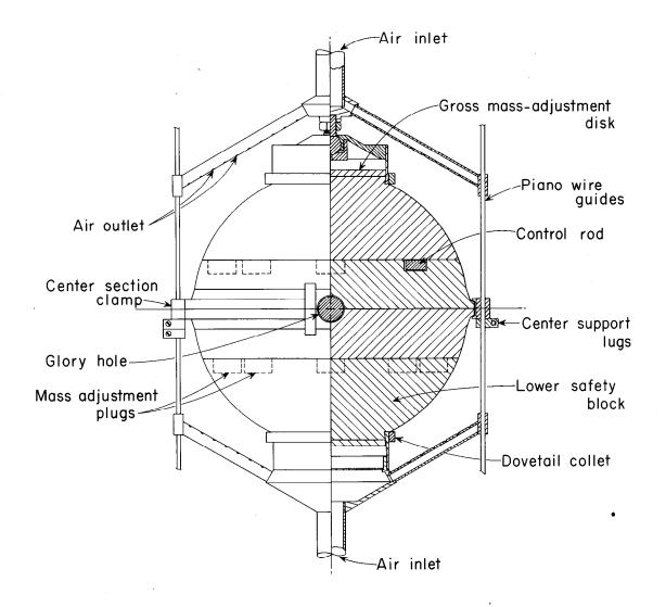
Fig. 5. The active portion of original Jezebel, the bare plutonium assembly. Cooling air blows out of the locating arms that ride on taut wires.
