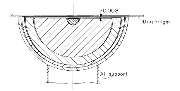
Fig. 3. Exaggerated defect of the shell model shown in Fig. 2; gaps on the parting plane are introduced by lower shells in contact.
