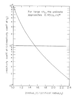
Fig. 4. Relative contributions of external material to the reactivity of a critical bare sphere. Measured values near the sphere surface connect smoothly with the r<sup>-4</sup> relation that applies to objects of limited size at large distances r.
