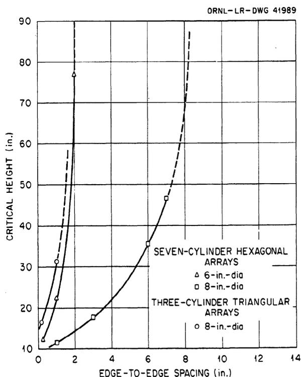
**Fig. 3.7.1. Critical Solution Height as a Function of Edge-to-Edge Spacing of Unreflected Triangular and Hexagonal Arrays of 6- and 8-in.-dia Aluminum Cylinders Containing Aqueous Solutions of 93.2% U<sup>235</sup>-Enriched Uranyl Fluoride (H:U<sup>235</sup> Atomic Ratio = 309).**
