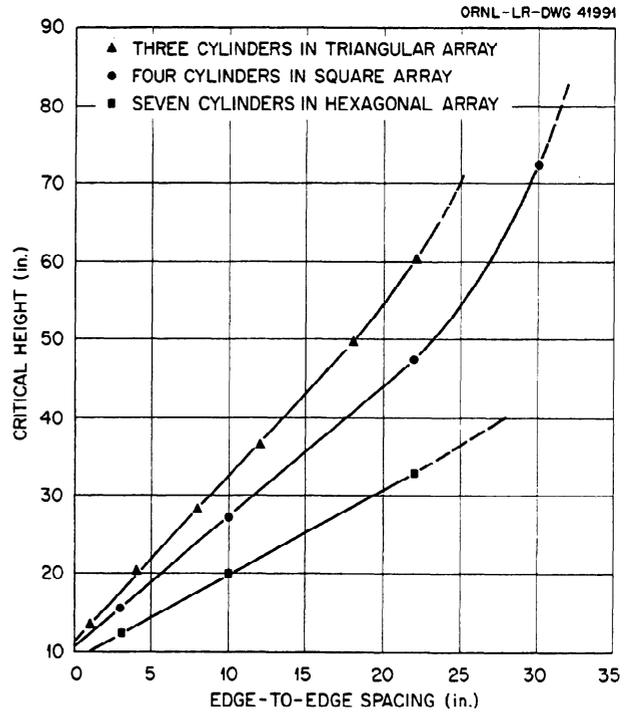
Fig. 3.7.3. Critical Solution Height as a Function of Edge-to-Edge Spacing of Unreflected Triangular, Hexagonal, and Square Arrays of 9.5-in.-dia Aluminum Cylinders Containing Aqueous Solutions of 93.2%  $U^{235}$ -Enriched Uranyl Fluoride (H: $U^{235}$  Atomic Ratio = 297).
