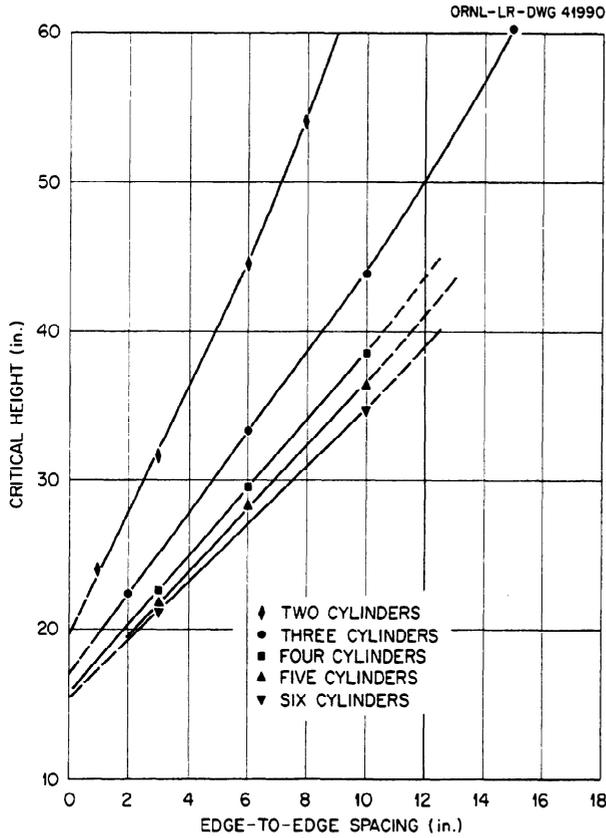
Fig. 3.7.2. Critical Solution Height as a Function of Edge-to-Edge Spacing of Unreflected Straight-Line Arrays of 9.5-in.-dia Aluminum Cylinders Containing Aqueous Solutions of 93.2%  $U^{235}$ -Enriched Uranyl Fluoride (H: $U^{235}$  Atomic Ratio = 297).
