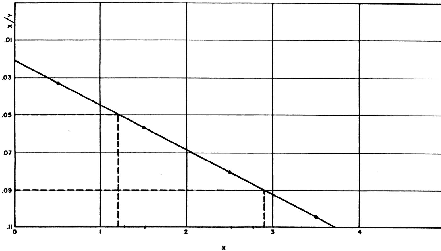
$$\text{SLOPE} = \frac{\Delta X/Y}{\Delta X}$$
