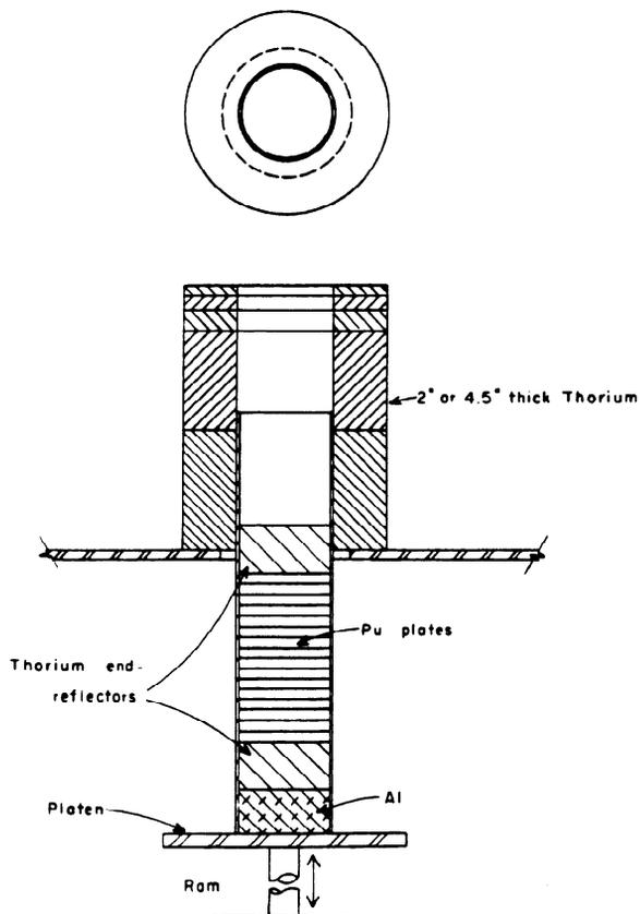
FIG. 3. Setup for reflected measurements of dilute Pu cylinders on assembly machine.
