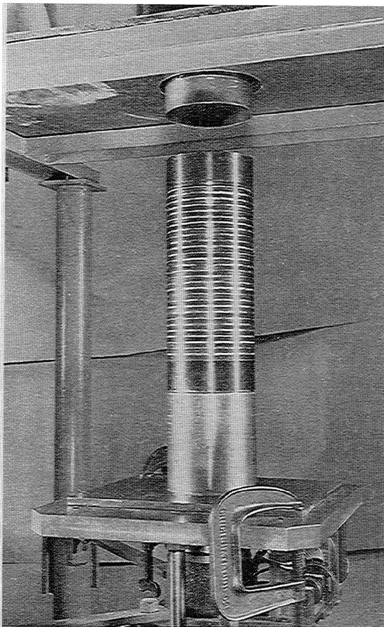
FIG. 2. Dilute Pu cylinder ( $\text{Pu}:\text{U}^{238} = 1:2$ ) stacked on lift with 2-in. thick reflector cylinders on top and bottom of core.
