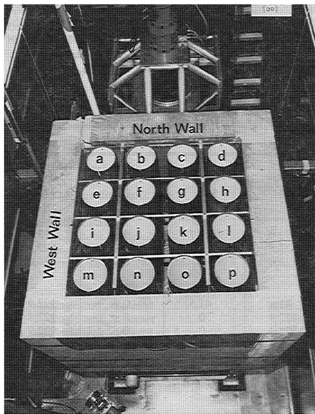
Fig. 3. An array of cylinders in the concrete reflector.
