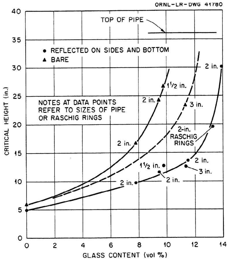
**Fig. 3.6.1. Critical Heights, as a Function of the Pyrex Content, of Bare and Reflected 20-in.-dia Stainless Steel Cylinders Containing a Pyrex-Poisoned Aqueous Solution of 87.4% U<sup>235</sup>-Enriched UO<sub>2</sub>(NO<sub>3</sub>)<sub>2</sub>.**
