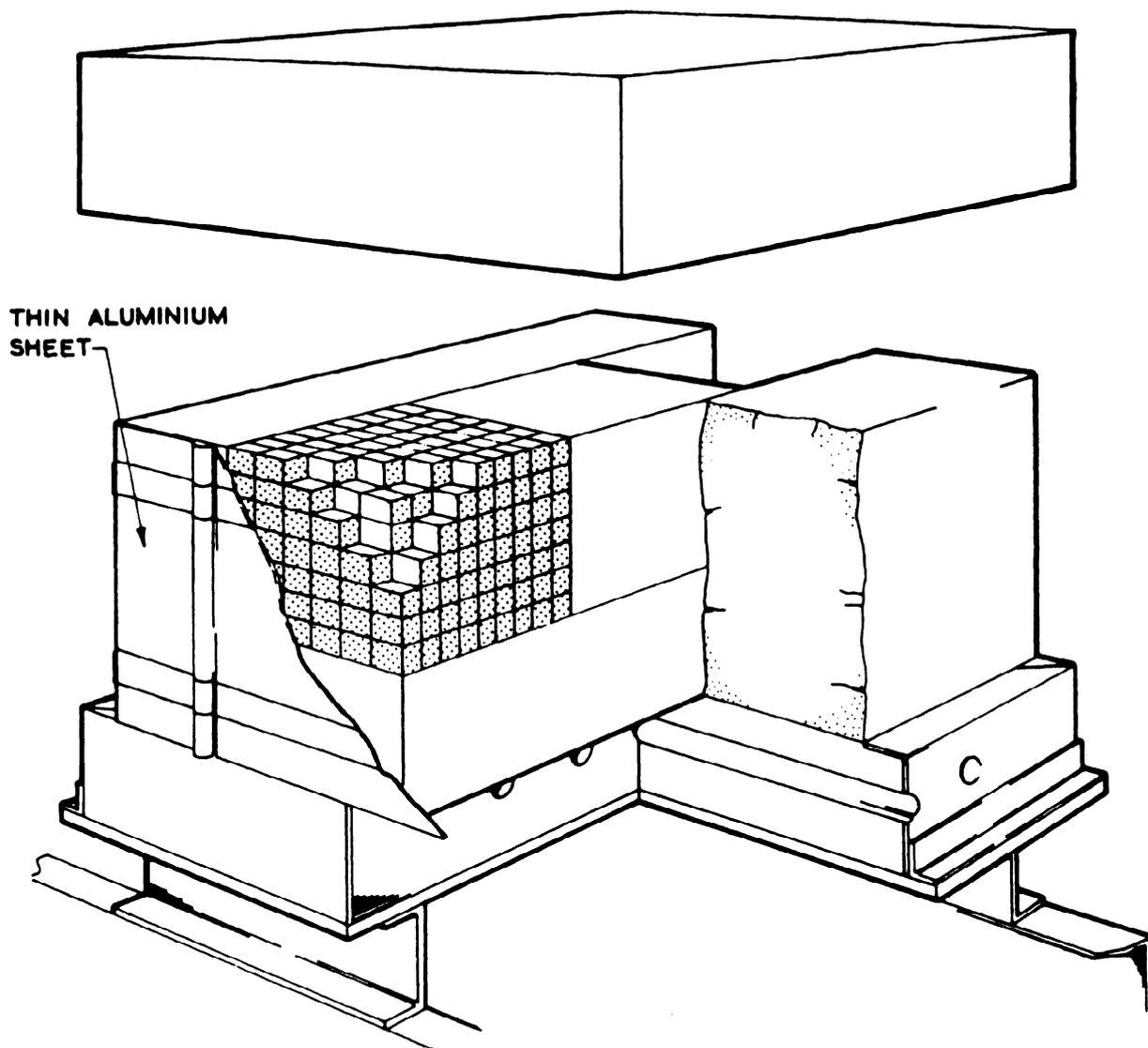
FIGURE 6. CORE AND REFLECTOR ARRANGEMENT FOR
