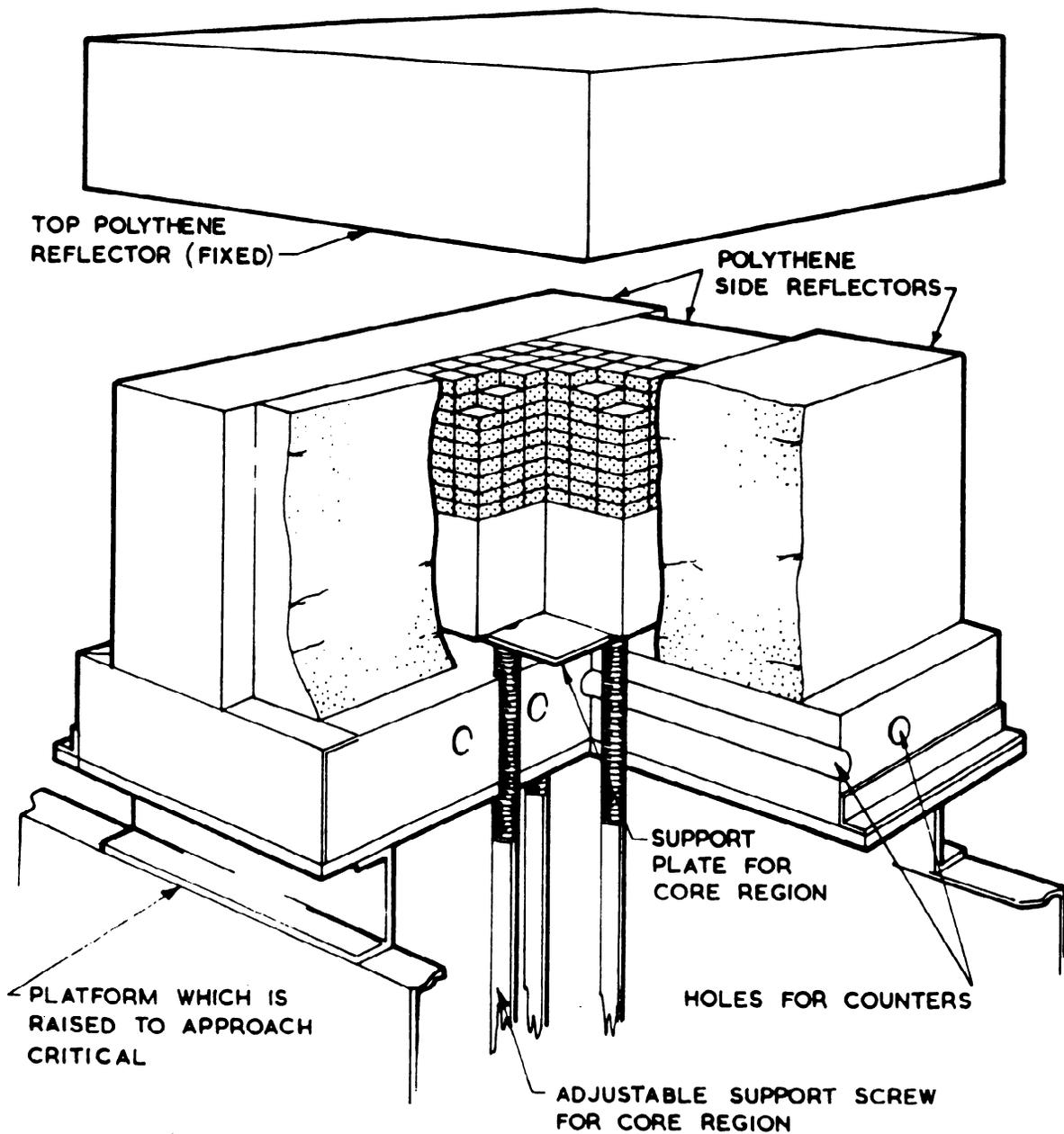
**FIGURE 4. CORE AND REFLECTOR ARRANGEMENT FOR FULL POLYTHENE REFLECTION**
