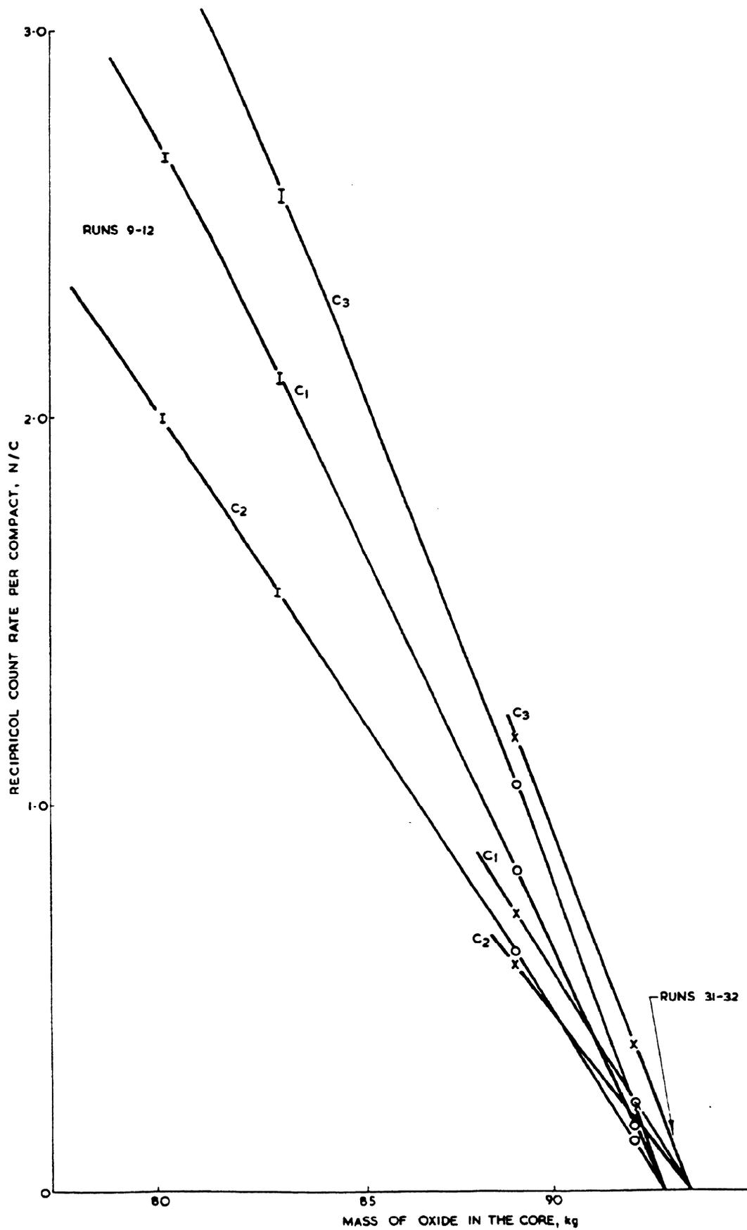
FIGURE 7. EXTRAPOLATION TO CRITICAL FOR CORE HAVING 25.7cm X 25.7cm BASE
