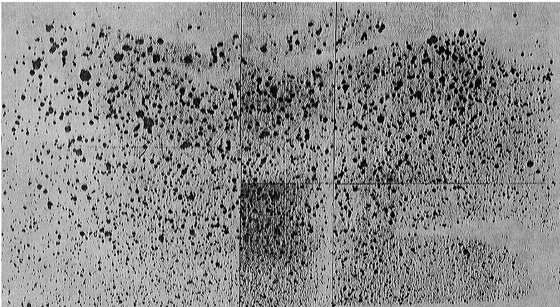
FIGURE 2. RADIOGRAPH OF UO<sub>2</sub>/POLYTHENE COMPACT
