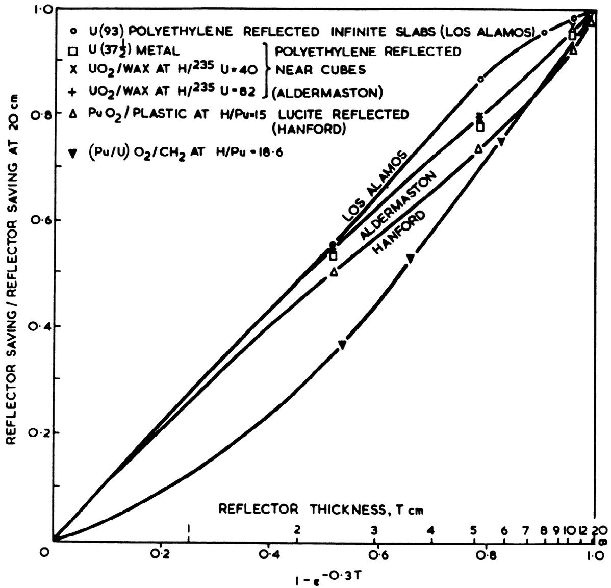
FIGURE 12. VARIATION OF REFLECTOR SAVING WITH THICKNESS
