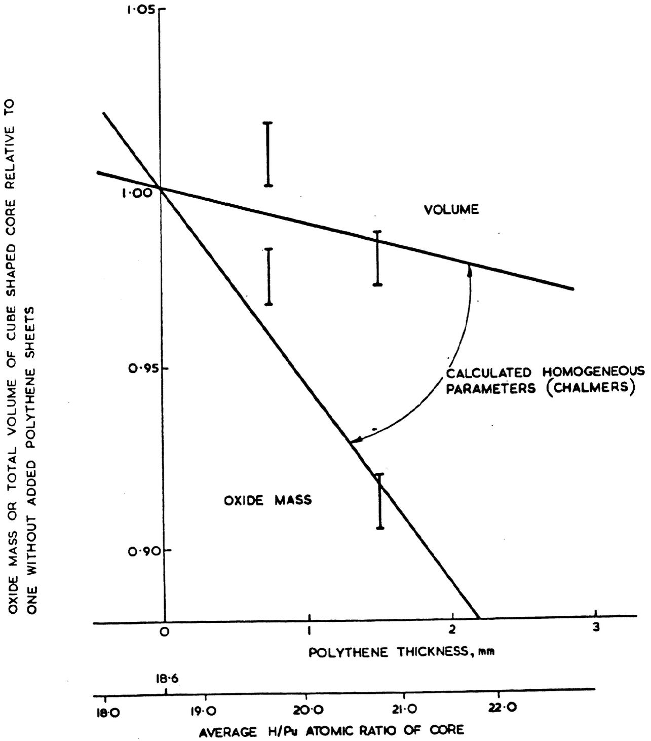
FIGURE 13. EFFECT OF ADDING POLYTHENE SHEETS TO A CORE ON ITS CRITICAL PARAMETERS
