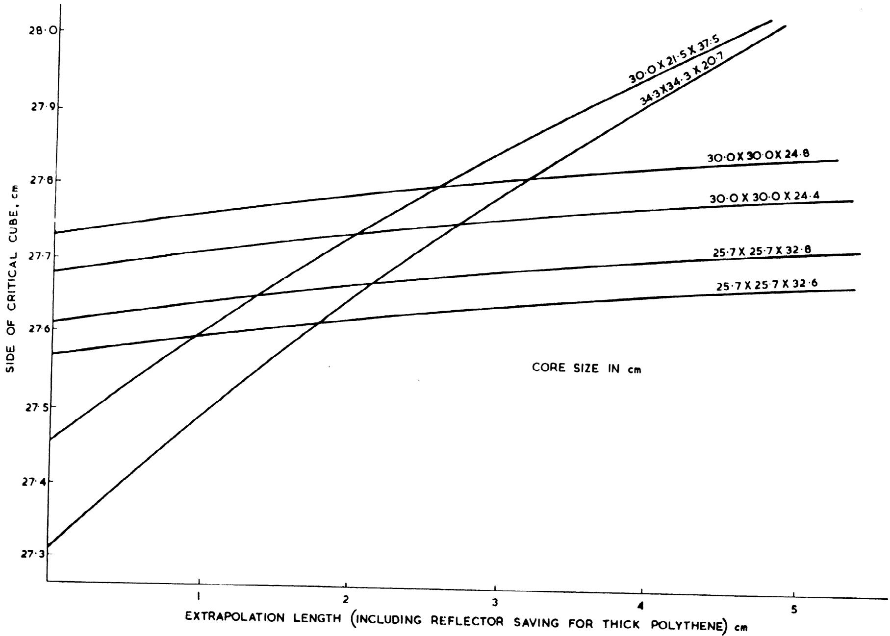
FIGURE 10. BUCKLING CONVERSION OF THICK POLYTHENE REFLECTED CRITICAL PARALLELOPIPEDS TO CUBE GEOMETRY
