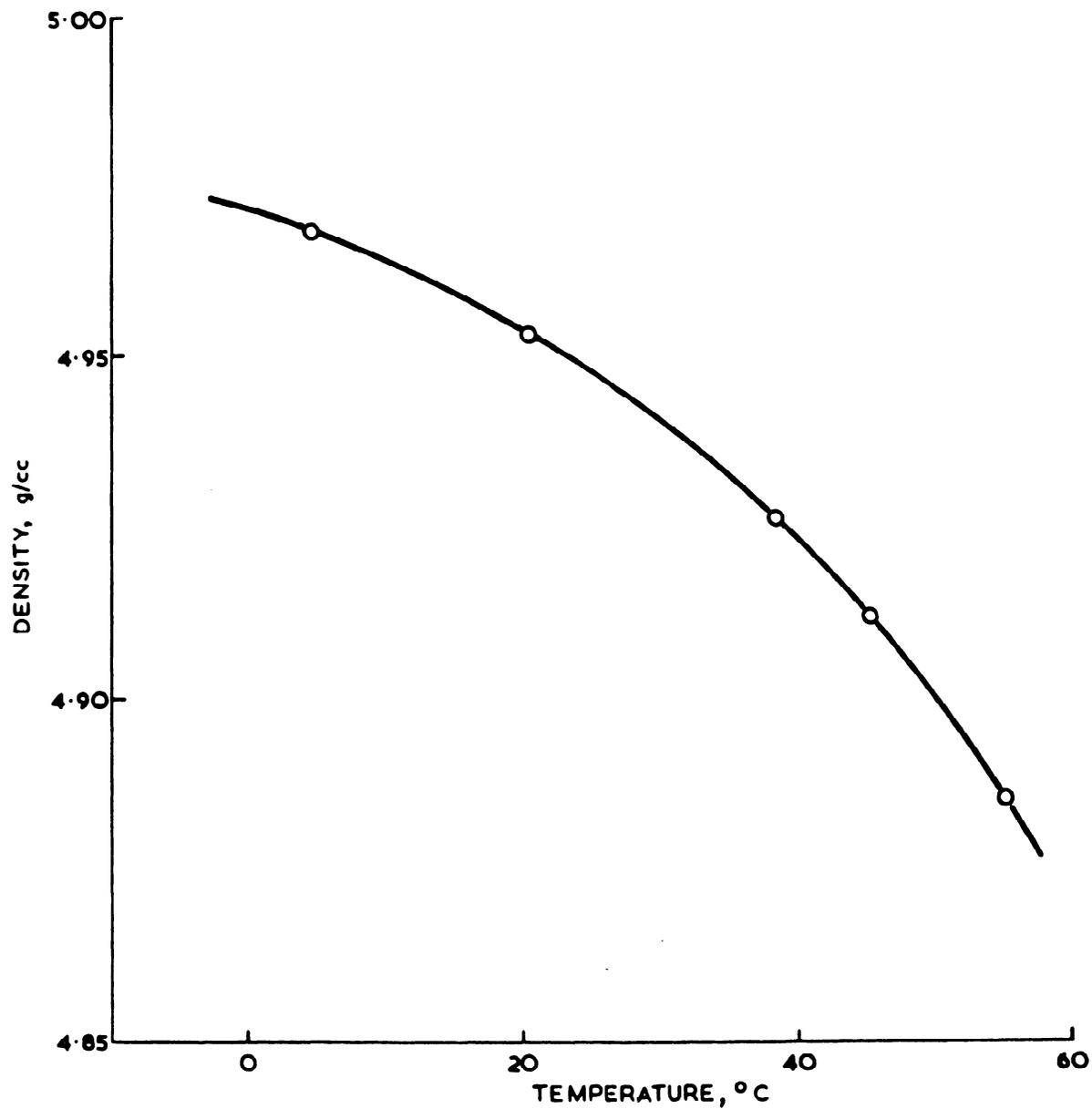
**FIGURE 3. CHANGE OF DENSITY WITH TEMPERATURE FOR A PARTICULAR COMPACT**
