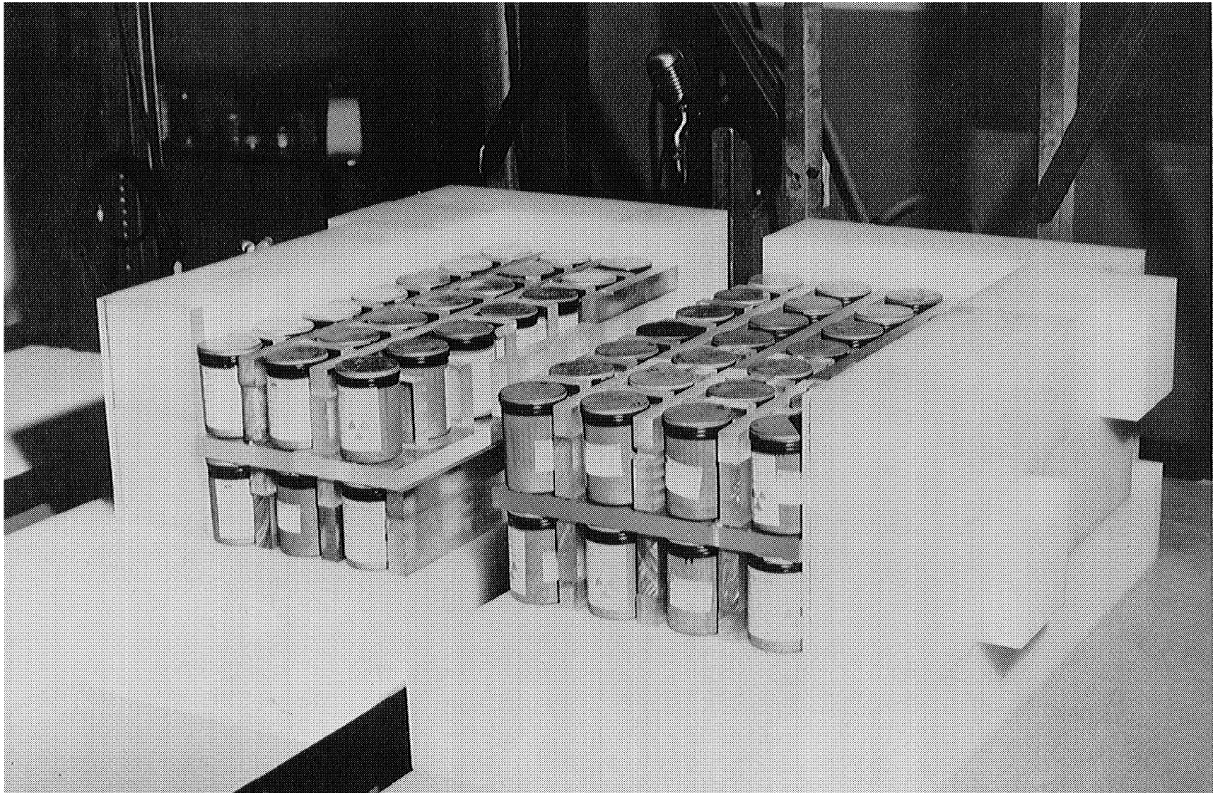
Fig. 1. Photograph of a 7 \times 7 \times 2 Array of 421 g Fissile Units of UO_2 .
