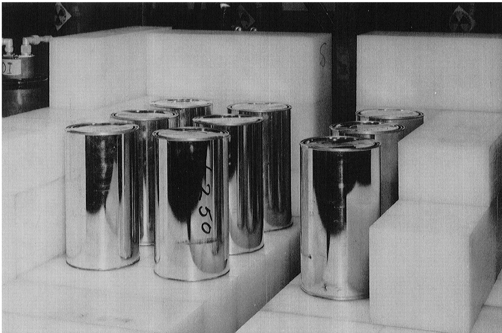
Fig. 5. Photograph of a 3 \times 3 \times 1 Array of 17 kg Fissile Units of UO_2 -Alcohol.
