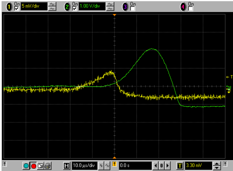
Figure 4.11. A preamplifier waveform from the noncollecting anode (yellow) and the shaped signal (green). The shaping time used is 16 \mu\text{s} .
