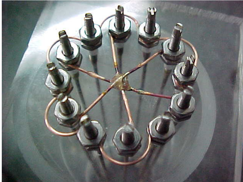
Figure 4.1. A photograph of the anode structure in a test assembly. The connection scheme used to group the wires into two signal electrodes is apparent.
