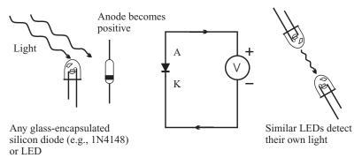
**Figure 1.3** Any diode, even a silicon rectifier, can show photosensitivity if the light can get to the junction. LEDs generate higher open circuit voltages than the silicon diode when illuminated with light from a similar or shorter wavelength LED.
