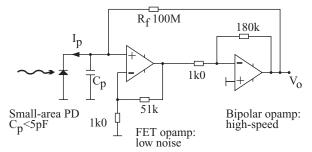
**Figure 2.10** Transimpedance receiver with loop gain shared between two different amplifiers. This can improve bandwidth for high parasitic capacitance photodiodes. (*Courtesy of Robert Theobald of Theoptics Ltd.*)
