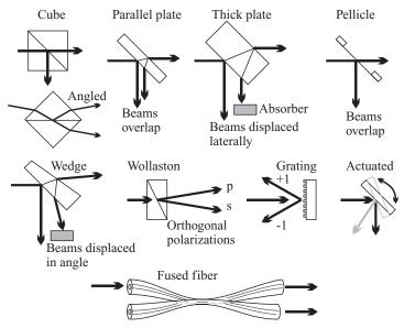
Figure 8.13 Selection of beam-splitters used for intensity referencing.
