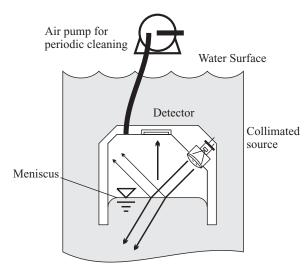
**Figure 9.12** Free surfaces within the bulk of a liquid sample are possible using an inverted-cup. Occasional pressurization with a surface air-pump will clean away accumulated debris.
