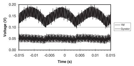
**Figure 7.7** Response of the circuit of Fig. 7.6 to 50 Hz fluorescent lighting and a 10 kHz modulation. The 100 Hz rectified sine wave of the upper response is almost suppressed with the active feedback circuit shown in the lower curve.
