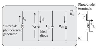
**Figure 1.7** A photodiode can be modeled as a current generator proportional to the incident light intensity in parallel with an ideal diode, a shunt resistance, and a shunt capacitance. These significantly influence the diode's performance, depending on the external circuitry.
