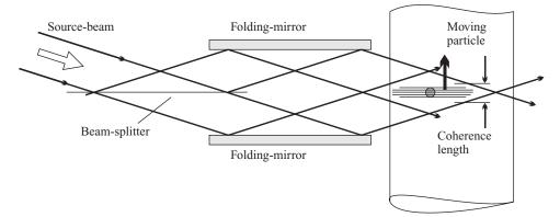
Figure 7.18 Low coherence-length sources can be used to localize the interference pattern in a confined region.
