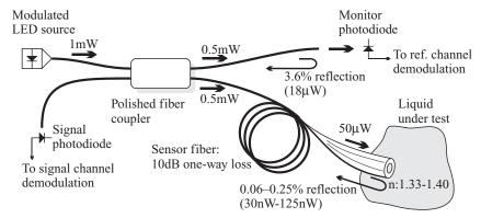
**Figure 8.23** Measurement of changes in power reflected back from a distant fiber end is attractive for a wide variety of sensing applications. However, performance is severely compromised by changes in fiber loss, or by the more intense reflection from a monitor-photodiode branch. The simple configuration is unusable except in the most benign environments.
