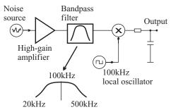
**Figure 3.19** Flat noise sources can be obtained by frequency shifting high-frequency noise using the multiplier of a lock-in amplifier.
