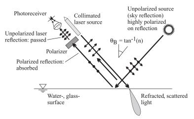
**Figure 7.12** Polarizers can be useful to suppress highly polarized interfering sources, for example from daylight reflections off surfaces close to Brewster's angle. This example is from a laser-based water turbidimeter for outdoor use.
