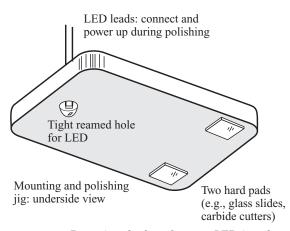
Figure 6.13 Removing the lens from an LED is a fiveminute job if you have a polishing jig. A "three-point" support gives quick and controllable results. Ideally, power up the LED during polishing to be sure you haven't planed off the wire-bond!
