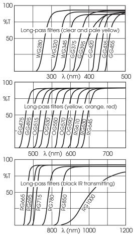
**Figure 7.10** Examples of colored glass filter responses. Edge filters are available with modest slopes and very strong blocking of out-of-band wavelengths. These are very useful for many instrument applications. Figure supplied and reproduced by permission of Comar Ltd, Cambridge U.K.
