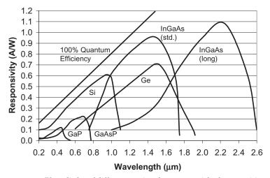
Figure 1.5 Photodiodes of different semiconductor materials show sensitivity in different wavelength regions, limited at long wavelength by their energy gap. 100 percent quantum efficiency means that one photon produces one hole-electron pair.
