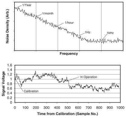
**Figure 10.16** Logged instrumentation data suggest that the "noise-and-drift" power spectrum is not white, but increases at low frequencies, giving errors far greater than expected from the instrument's optical noise performance. The time-series was calculated using a 1/f power spectrum, and looks like real data. The greater the period between calibration and operational use, the greater the measurement variance.
