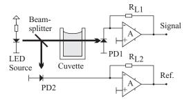
**Figure 8.10** Optical referencing can reduce the requirements on LED output stability and greatly improve overall transmission measurement stability. However, the photodiodes must track with temperature, and "asymmetric" window contamination must be kept to a minimum.
