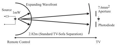
Figure 3.5 An example of an optical communication system: the TV remote control.
