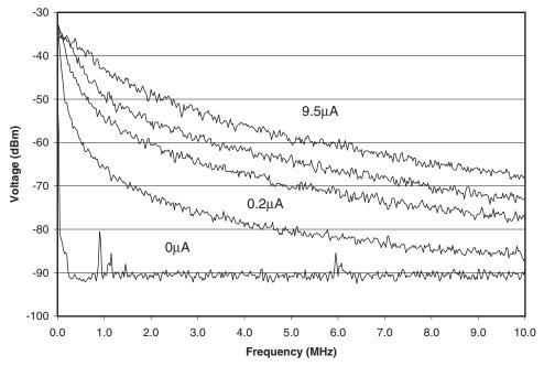
Figure 3.22 Frequency spectrum of the ZTX453 noise generator at current (bottom to top) of 0, 0.2, 1.1, 2.95,  $9.5 \,\mu$ A.
