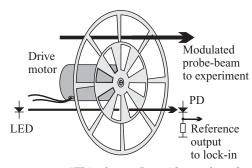
**Figure 5.19** "Thin chopper" provides weak modulation at both even and odd harmonics of the fundamental. A separate reference channel allows use with a conventional lock-in amplifier.
