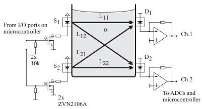
**Figure 8.20** Four-beam configuration. By measuring transmission intensities along the four paths  $L_{ij}$ , the absorption coefficient of a uniform material can be determined even with slow changes in source output and detector responsivity.
