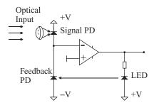
**Figure 4.2** An optical feedback transimpedance amplifier.
