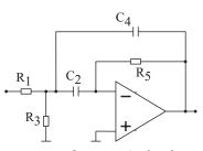
**Figure 3.15** Narrow-band filters are useful to estimate the noise at one spot-frequency. The quasisinusoidal output can be quantified using a scope or AC voltmeter.
