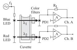
**Figure 11.2** Multiple channels can be separated spatially and with matched color filters.
