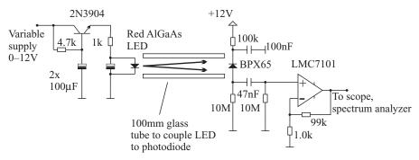
**Figure 3.7** Another shot-noise demonstrator. A quiet current source drives the LED. An optical waveguide increases optical coupling efficiency without increasing electrical interference coupling.
