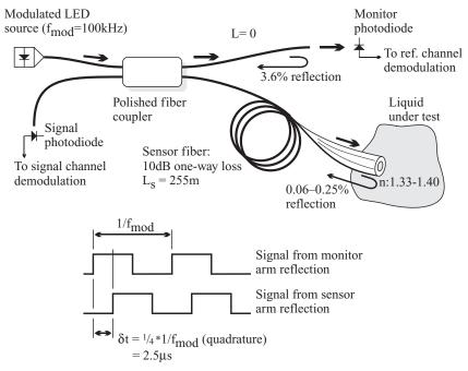
**Figure 11.6** Phase-coding applied to a long fiber reflectometer. The main reflections from the sensor and from the reference arm can be arranged to be in quadrature through correct choice of the source modulation frequency.
