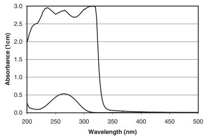
**Figure 7.11** Absorbance spectrum of dilute and strong solutions of acetone in water. Many chemicals have useful filter responses, especially edge filters in the UV. Their great advantages are strong blocking, easy absorbance adjustment, and shape flexibility.
