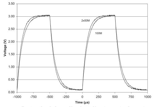
Figure 2.16 Experimental results for a 100-M $\Omega$  and  $2 \times 50$ -M $\Omega$  resistor transimpedance receiver.
