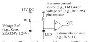
Figure 8.5 The terminal voltage of the source LED itself provides an effective local temperature measure. The LED current should be stabilized to high precision with a current source or voltage reference and low tempco resistor.
