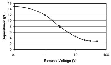
**Figure 2.4** Photodiode capacitance is a function of reverse bias voltage. Values for a BPX65 are shown. High voltage will increase detection bandwidth at the expense of increased dark leakage current.
