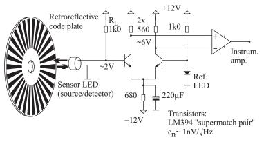
**Figure 4.5** An LED can be used both as a source and simultaneously as a detector of its own light, for example to detect a rotating reflective encoder. For low-noise detection the transistor amplifier must be chosen for lowest  $e_n$ , lowest base spreading resistance  $r_{bb}$ , and high collector current.
