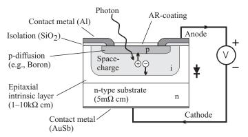
**Figure 1.4** Most photodiodes are formed by diffusing dopants into epitaxially formed layers. The use of a low conductivity intrinsic layer leads to thickening of the space-charge region, lower capacitance, and improved sensitivity.
