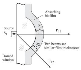
Figure 9.3 Domed windows can equalize the absorbing film atternuations, but at the risk of greater speed of contamination growth.
