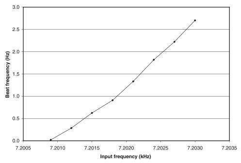
**Figure 5.23** Results of beat-frequency measurements obtained using a crystal controlled source modulator and a finely variable reference clock. The beat was easily visible on the lock-in's analog display.
