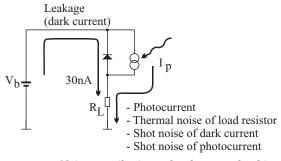
Figure 3.3 Noise contributions of a detector plus bias box.
