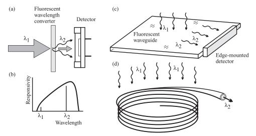
**Figure 4.8** Wavelength conversion can improve detection sensitivity in regions of poor photodiode responsivity. Fluorescent and scintillating materials can be formed into face plates, planar waveguides, and fibers.
