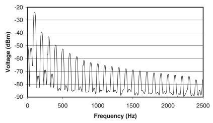
**Figure 5.5** Measured frequency spectrum of a photodetector illuminated by 50 Hz fluorescent lighting, showing harmonics of 100 Hz out to 2.5 kHz.
