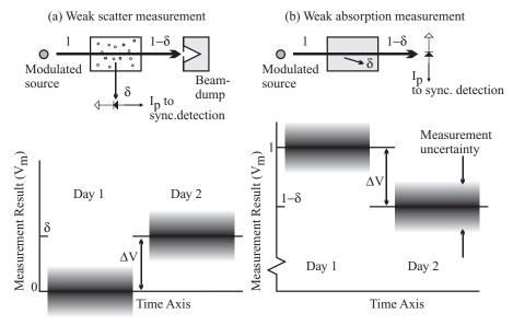
**Figure 10.1** Dark-field detection, for example of low levels of optical scatter (a), is limited by noise and spurious scatter from the sample cell. Weak absorption measurements (b) are additionally limited by changes in source intensity and detection scale-factor.
