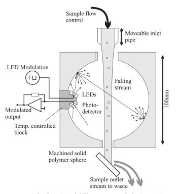
**Figure 9.18** Combination of falling stream and the integrating sphere makes possible noncontact absorption measurement with reduced sensitivity to attenuation by scatter. Absorption depends only on the volume of liquid, not the shape. Individual drops work fine.
