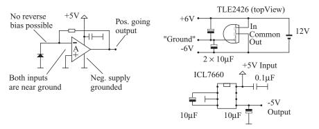
**Figure 6.11** Single-supply operation of transimpedance amplifiers is possible, although performance may suffer. Bipolar supplies may be obtained with artificial ground generators (TLE2426) or a switched-capacitor voltage inverter (ICL7660 and equivalents).
