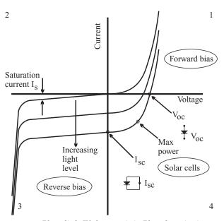
Figure 4.4 Photodiode IV characteristic. Photodetection is possible in quadrants 1, 3, 4.
