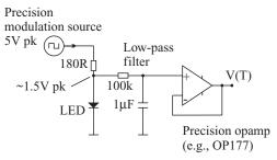
**Figure 8.6** Temperature estimation of a modulated LED is also possible by smoothing (or synchronously detecting) the terminal voltage variations.
