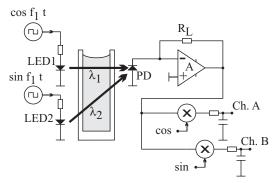
Figure 11.5 Phase-coding of two measurement channels.
