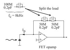
**Figure 2.14** Bandwidth-limiting effects of the parasitic capacitance present in all resistors can be reduced by splitting the resistor into two components of half the value.
