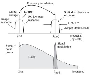
Figure 5.2 The synchronous demodulator effectively translates the single-sided low-pass filter characteristic out to a symmetrical response centered on  $f_{\rm mod}$ .
