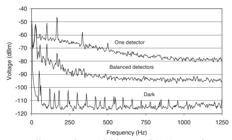
Figure 8.17 Noise spectra of a  $1.55\,\mu\text{m}$  diode laser source illuminating just one detector, or two detectors arranged for equal photocurrents. The shot noise level at this photocurrent is  $-98\,\text{dBm}$ .
