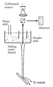
**Figure 9.17** Axial propagation in a falling liquid thread is useful for non-contact scatter, fluorescence and Raman detection.
