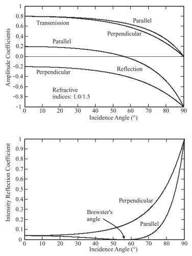
**Figure 7.13** The amplitude and power reflection coefficients are given by the Fresnel equations. At Brewster's angle the reflection coefficient for parallel-polarized light vanishes, giving a highly polarized reflection.
