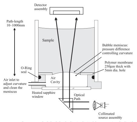
**Figure 9.15** Better control of the holey bucket is obtained by supporting the liquid column primarily on a pressurized air cushion. The meniscus curvature may be adjusted using feedback control from the differential pressure. Plane menisci are possible, or we can make use of the optical power of a curved liquid surface for beam collimation.
