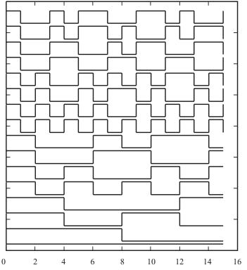
Figure 5.12 The 16-bit Walsh function waveforms.
