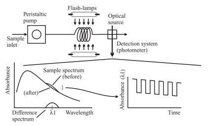
**Figure 10.10** In-situ flash photolysis is a technique to modulate the optical absorption of a photo-active species in a complex nonactive matrix. Subtraction of the before/after spectra reduces the effects of absorbance drifts due to the matrix.
