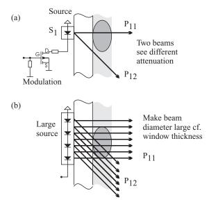
Figure 9.4 Contamination of just the "wrong size" reduces the effectiveness of multibeam compensation (a). Sources and detectors which are large with respect to the contamination granularity can help (b).
