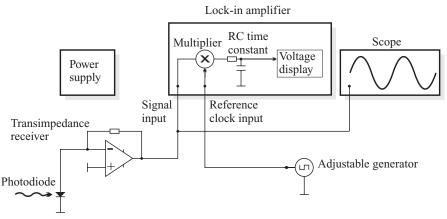
Figure 5.21 With an adjustable reference frequency, different frequency components present in the input can be detected. The system is a slow spectrum analyzer.
