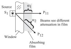
**Figure 9.2** Fouling layers are not completely compensated by the four-beam technique, as the different beams see different layer thicknesses and attenuations.
