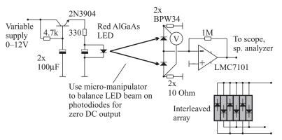
**Figure 3.27** Two-photodiode shot-noise generator. By balancing the two photocurrents the opamp output is at zero volts but shows the added noise power of the two photocurrents. An illuminated interleaved isolated diode array might be a useful noise source.
