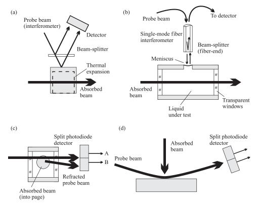
**Figure 4.10** Optical absorption detection by (a) thermal expansion of a solid, (b) thermal expansion of a liquid, (c) refractive index changes in a liquid, and (d) in a gas (mirage effect).
