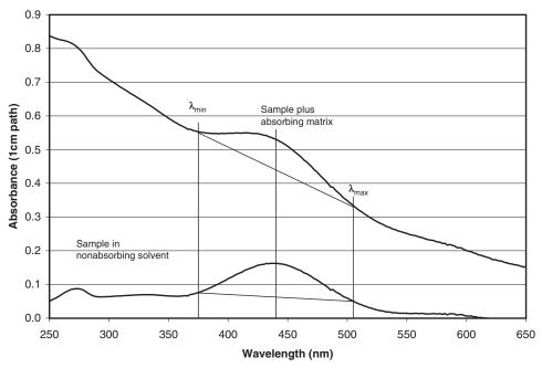
**Figure 9.7** Where the known absorption feature is added to a nonuniform absorbing background, three-point measurements can help to recover the true absorbance. Calculate at the peak, or find the area under the feature.
