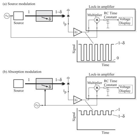
**Figure 10.2** Source modulation (a) does little to improve the weak absorbance measurement, as the minimum detectable transmission change is defined by the source/detection stability. If the absorbance itself can be modulated (b), much smaller transmission changes can be detected.
