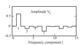
Figure 5.13 Walsh frequency spectrum of a sine wave.
