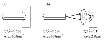
Figure 2.5 Careful alignment of single-mode optical fibers allows the use of photodiodes with very small areas (<30  $\mu m$  diameter). Increasing the numerical aperture (NA) of the incident light in principle allows the use of even smaller detectors.
