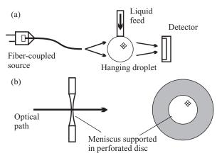
**Figure 9.13** Small liquid samples may be supported by surface tension and probed in transmission without use of wetted windows, either using hanging droplets or a thin film.
