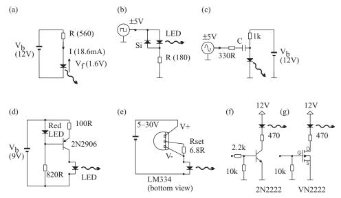
**Figure 6.2** LED drive circuit fragments. As the LED is a diode, it is more comfortable to define the LED current and let the voltage take on whatever value it needs. (b) and (c) show square wave and sine wave modulation schemes. (d), (e) are simple DC current generators. If more current is needed than an opamp or CMOS logic gate can supply, use a bipolar transistor or FET buffer (f,g).
