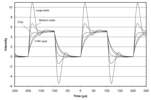
**Figure 2.13***a* Response of a transimpedance amplifier for a selection of 100-M $\Omega$  resistor types, including large plate types, 1/4-W axials and a chip types. The fastest response was obtained with a chip component.
