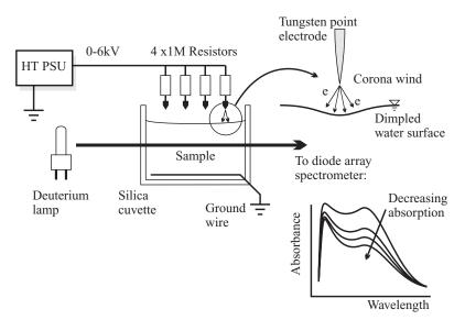
**Figure 10.12** Corona-wind modulation spectroscopy. Charged particle injection from a high-voltage corona can be used to degrade and modify a wide variety of organic samples. The system is easily installed within the measurement spectrometer.
