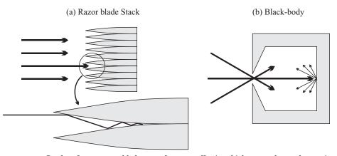
**Figure 7.16** Stacks of new razor blades can form an effective, high power beam dump via multiple reflections and absorptions. A small aperture in a large, diffusely reflecting cavity also works well.
