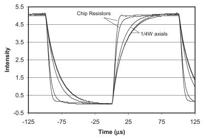
**Figure 2.13***b* Detailed view of the transient response. The slowest responses are for a 1/4-W axial resistor, the two fastest for a chip component wired "casually" and in an optimized compact construction.
