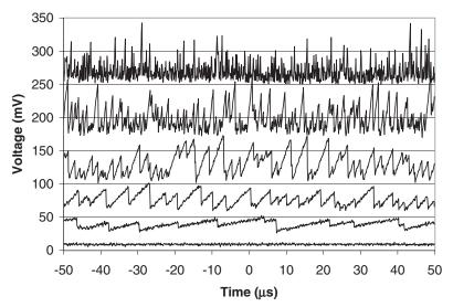
Figure 3.21 Time response of the ZTX453 noise-generator. From bottom to top the reverse DC current is 0, 0.2, 1.1, 2.95, 9.5,  $31.5\mu$ A. Increasing current increases the noise bandwidth.
