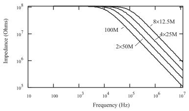
Figure 2.15 Calculations of the frequency-variation of impedance for a  $100\,M\Omega$  resistor split 2, 4, and 8 ways.
