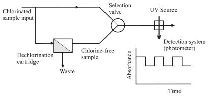
**Figure 10.9** A useful technique is to derive the absorbance-free reference liquid from the sample itself, for example via dechlorination.
