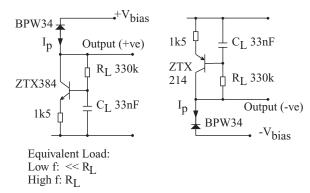
**Figure 7.4** A nonlinear transistor load can synthesize the operation of an inductor, with excellent suppression of DC and low-frequency light. Low frequency photocurrents forward bias the transistor and short out the load resistor. Circuit reproduced by permission of Zetex Ltd.
