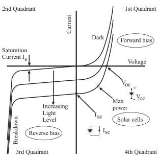
**Figure 1.9** Four-quadrant current/voltage characteristic. Without illumination this is similar to a conventional diode. Increasing illumination shifts the characteristic in the negative current direction. Detection is possible in quadrants 1, 3, and 4.
