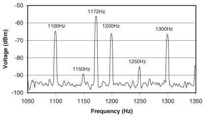
Figure 5.6 Positioning the modulation frequency (1172 Hz) between the interfering harmonics can greatly improve S/N measurement. Hitting a harmonic would degrade S/N by about 25 dB.
