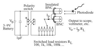
**Figure 2.1** The bias box uses a small battery to reverse bias a photodiode and pass its photocurrent through a choice of load resistors. It is a simple, useful detector. Changing the resistor allows a trade-off between output voltage and detection speed.
