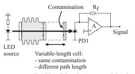
**Figure 10.3** Variable cell-length gives a modulated intensity, with slow changes due to window contamination compensated.
