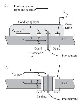
**Figure 2.3** Guarding using printed electrodes can only protect against surface currents (a). Currents may also flow in the bulk of the printed circuit board and in any conducting layer. The calculation of the currents requires a 3D model. Fully coaxial guarding (b) can additionally reduce PCB currents.
