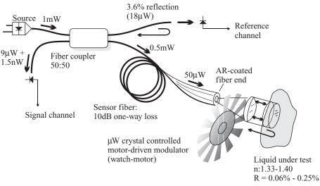
**Figure 10.15** Clockwork, battery, solar or fiber-powered modulators placed at the point of measurement are useful to aid the determination of weak intensity reflection changes, which would otherwise be swamped by fiber loss variations and spurious reflections from other fiber components.
