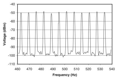
Figure 3.26 High-resolution view of the individual PRBS frequency spectrum lines, here separated by  $6.41\,\mathrm{Hz}$ .
