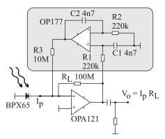
**Figure 7.6** The integrator in the active feedback loop also suppresses low frequency response, but maintains signal linearity. Circuit reproduced by permission of Texas Instruments Burr-Brown.
