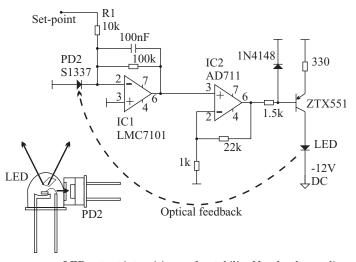
**Figure 8.12** LED output intensities can be stabilized by closely coupling source and reference photodiode, e.g., by gluing, and using a simple analog feedback controller.
