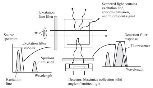
**Figure 4.9** Sensitive detection of fluorescence requires well-defined wavelengths of excitation and detection. This generally requires both source filters (to remove fluorescence wavelengths) and detection filters (to remove the source light wavelengths).
