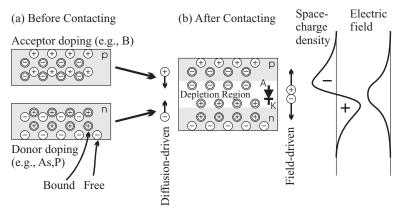
**Figure 1.1** The pn-junction. The presence of predominately different polarities of free carriers in the two contacted materials leads to asymmetrical conductivity, a rectifying action. Bound charges are indicated by a double circle and free charges by a single circle.
