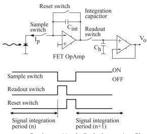
**Figure 4.3** Purely capacitive feedback photoreceiver. Photocurrent is integrated on  $C_{int}$ , and then read out using logic driven switches. Adapted from Liu et al. (1993).
