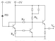
**Figure 2.12** The highest speed transimpedance amplifiers are often simple circuits made with heavily reverse-biased, specially selected low capacitance photodiodes and high GBW discrete semiconductors.
