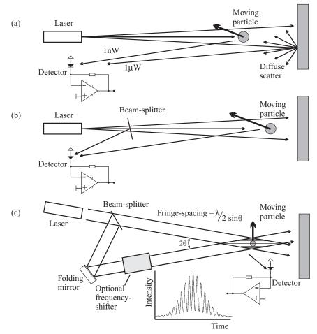
**Figure 7.17** Where intense scatter is unavoidable, source modulation is little help (a). Coherent detection effectively modulates the received signal depending on the particle's velocity (b). (c) An alternative configuration which allows more flexible choice of the modulation frequency.
