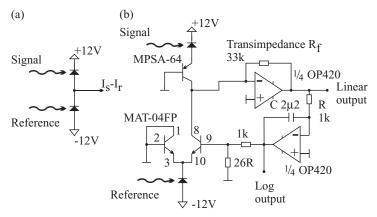
**Figure 8.18** Signal and reference currents can be automatically subtracted using this elegant circuit fragment. A feedback loop adjusts the proportion of the reference photocurrent that is subtracted from the signal to give zero. This allows intensity noise suppression right down to the shot noise limit. Circuit reproduced by permission of PC.D. Hobbs.
