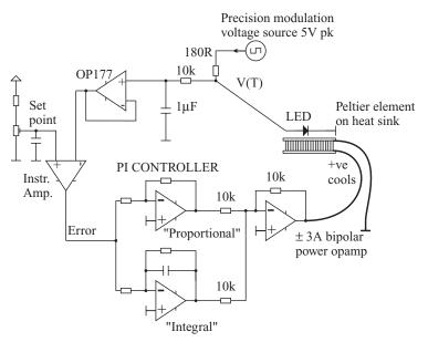
Figure 8.7 Precision temperature control of an LED source can be effected using a PI-controller and Peltier element heat pump. Temperature fluctuations of 1 mK are relatively easy,  $10 \mu \text{K}$  possible with care.
