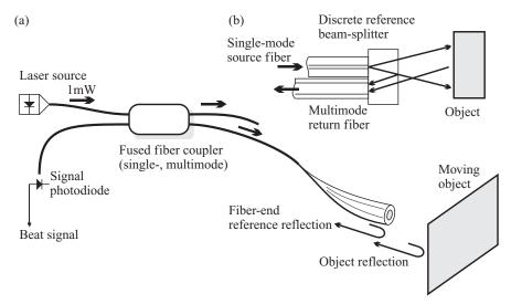
**Figure 7.19** By forming the interference with a reference reflection at the distal fiber end, the delivery fiber length is unimportant; even multimode fibers work well. However, speckle is still disturbing, so a singlemode fiber and tiny discrete beamsplitter can perform even better.
