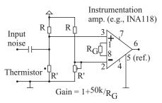
Figure 3.18 Waveform-independent noise power measurements can be made using heating of a thermistor to unbalance an electrical bridge.
