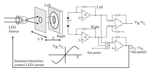
**Figure 8.19** Very simple but high resolution 1- and 2-dimensional position sensors can be fabricated using split (dual or quadrant) photodiodes illuminated by light from an LED, preferably cleanly apertured. The photocurrent difference gives the position, while the sum can be used to control the source intensity. Remanent scale factor errors occur if the axial separation Z changes.
