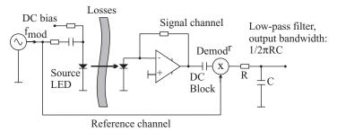
**Figure 5.1** Synchronous detection requires a reference signal that is phase-synchronous with the signal light and that is multiplied by the received signal. The combination of modulator and low-pass filter forms a bandpass filter centered on  $f_{mod}$ .
