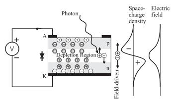
Figure 1.2 When a photon with energy greater than the material bandgap forms a hole-electron pair, a terminal voltage will be generated, positive at the p-type anode.
