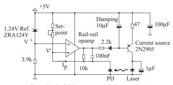
Figure 6.6 Example of a DC laser power-stabilization circuit.
