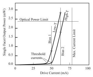
**Figure 6.4** Laser diodes exhibit a threshold characteristic. Normally we bias just above threshold and modulate with current pulses above. There are both maximum current and maximum power limits for each device and the threshold current, in particular, is temperature dependent. Correct biasing is simplest with feedback control from a monitor photodiode.
