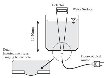
**Figure 9.14** *Holey cup.* Surface tension is useful to support macroscopic liquid samples above a small hole, allowing noncontact optical transmission measurements through large sample thicknesses.
