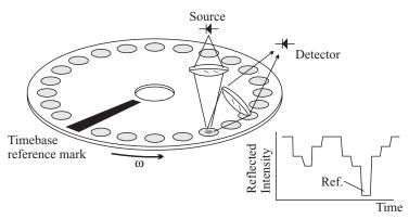
**Figure 10.14** Weak absorptions measured by diffuse reflectance can be detected at higher resolution by mechanically modulating the samples, spotted onto a uniform filter paper.
