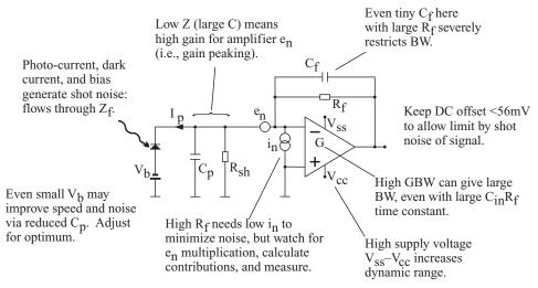
Figure 3.28 Summary of transimpedance design trade-offs for low noise and high bandwidth.
