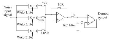
**Figure 5.15** Walsh modulator. Each binary multiplier is driven by one Walsh function, with the scaling gains applied in an analog gain stage. The result is equivalent to multiplication by a sine wave approximation.
