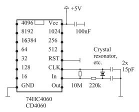
**Figure 6.9** The 74HC7060 provides a free gate for exciting crystal resonators, together with a long divider chain for selection of lower frequencies.
