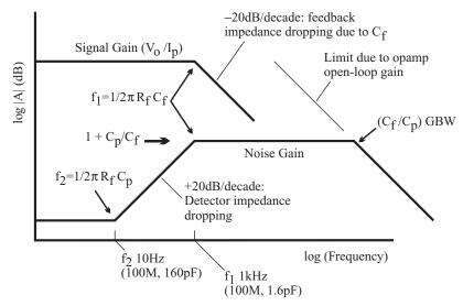
**Figure 3.10** Noise peaking. Signal gain is limited primarily by the transimpedance capacitance  $C_{f^*}$ . The amplified voltage noise  $e_n$  increases with frequency and can dominate the noise power for high-capacitance photodiodes with high-value transimpedance resistors.
