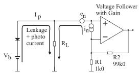
Figure 3.6 The opamp gain stage will increase signal levels but cannot improve the signal-to-noise ratio.
