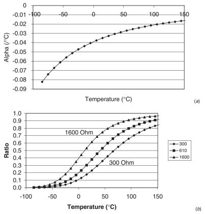
**Figure 8.3** (a) At room temperature the tempco of many thermistors  $\alpha$  is about -3.5 percent/°C. (b) The most linear region of a resistor/thermistor potential divider can be shifted though choice of the load resistor.
