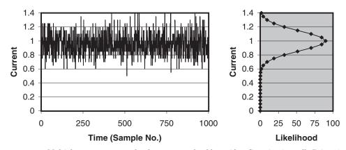
Figure 3.1 Multiple measurements of a photocurrent should provide a Gaussian (actually Poisson) histogram, with a variance equal to its mean.
