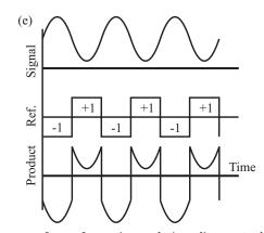
**Figure 5.3** Demodulator waveforms for various relative alignment phases. (a) in phase, (b) antiphase, (c) in "quadrature," (d) zero response to a DC signal, (e) DC-response removed, AC detected.
