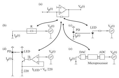
Figure 4.1 Alternative realizations of a resistor for use in transimpedance amplifiers.
