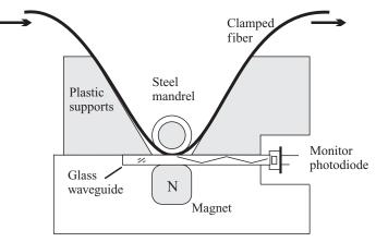
**Figure 8.15** Light can be tapped from a fiber using a small-radius bend. A magnet and steel mandrel make a convenient clamp, and even allow the light to be coupled to an embedded photodiode.
