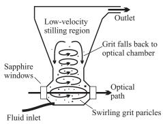
**Figure 9.9** Swirling grit particles or neutralbuoyancy plastic balls can be used to scour the cuvette windows to remove contamination, and yet be retained with little loss.
