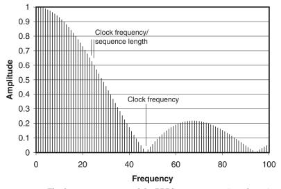
**Figure 3.24** The frequency spectrum of the PRBS generator consists of a series of lines separated by 1/(sequence repeat time), modulated by the sinc(x) waveform with its first null at the clock frequency.
