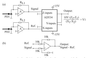
**Figure 8.16** Analog division of signal and reference is straightforward, but limited to about 1 percent precision, even at low frequencies. If signal and references are equal in magnitude, subtraction can offer higher precision and greater bandwidth.
