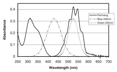
**Figure 11.1** The concentration of chemicals with well-defined absorbing and loss-less regions can be determined with high resolution by measuring at two wavelengths on and off the absorption feature and subtracting the absorbance values.
