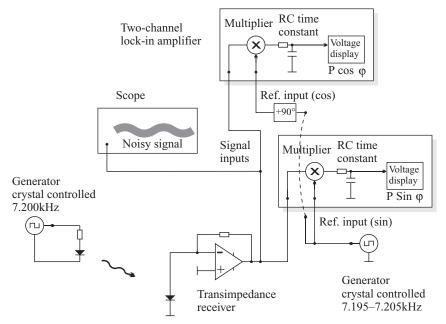
**Figure 5.22** The lock-in reference signal need not come from the source modulator. As long as the frequency difference is small enough to remain within the filter bandwidth, separate oscillators can be used. However, *two-phase* detection will be needed to measure the signal amplitude independent of drifting phase.
