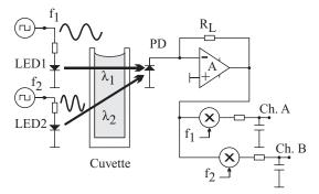
Figure 11.4 Frequency-coding of two or more measurement channels.
