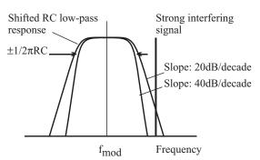
**Figure 5.20** Suppression of a strong interfering signal close to the modulation frequency can be obtained by narrowing the response (increasing the filter time-constant), by increasing the low-pass slope, or by increasing the separation from  $f_{mod}$ .
