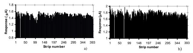
Fig. 4. a) Strip responses as measured at position A80; b) Strip responses as measured at position A20.
