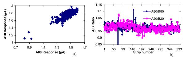
Fig. 5. a) A20 response versus A80 (for all strips) illustrates the uniformity at A20 and at A80 for all strips; b) Asymmetry across the strip (the strip number is not associated with production time).
