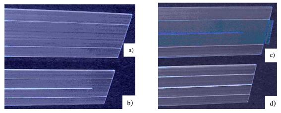
Fig. 1. a) A strip after extrusion; b) The same strip with a machined separation groove; c) The strip with blue tape; d) The trimmed strip with the glued separation groove.
